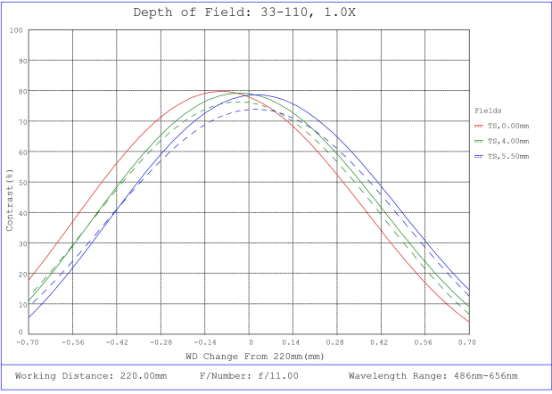
#33-110, 1X, 220mm WD, In-Line CompactTL™ Telecentric Lens, Depth of Field Plot, 220mm Working Distance, f11
