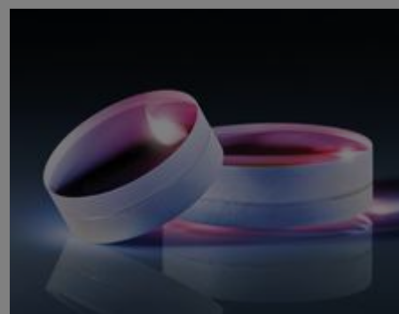
#32-311 - 12.5mm Dia. x 25mm FL, MgF 2 Coated, Achromatic Doublet Lens €86,00
