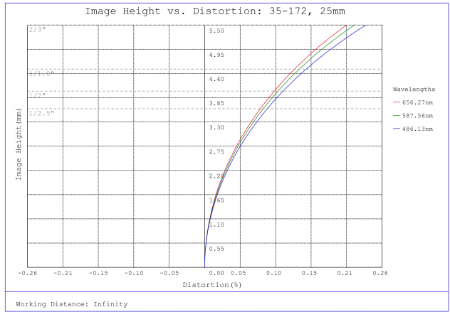
#35-172, 25mm, f/1.4 Cr Series Fixed Focal Length Lens, Distortion Plot
