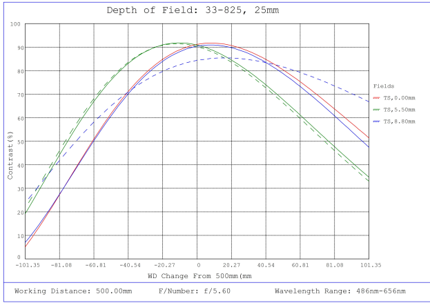
#33-825, 25mm f/5.6, HPI Series Fixed Focal Length Lens, Depth of Field Plot, 500mm Working Distance, f5.6
