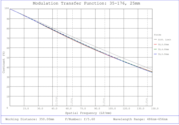
#35-176, 25mm, f/5.6 Cr Series Fixed Focal Length Lens, Modulated Transfer Function (MTF) Plot, 350mm Working Distance, f5.6
