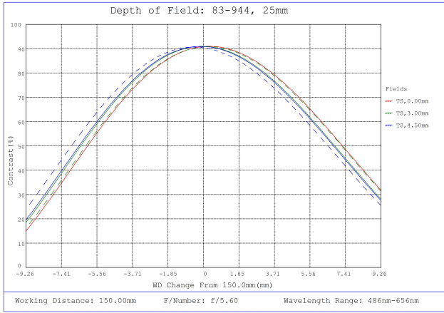
#83-944, 25mm FL f/5.6, Blue Series M12 Lens, Depth of Field Plot, 150mm Working Distance, f5.6
