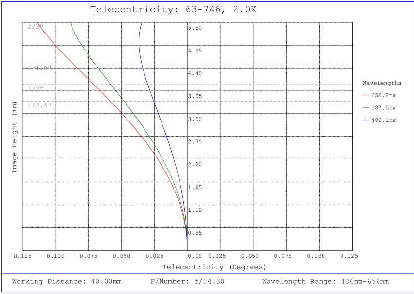
#63-746, 2X, 40mm WD CompactTL™ Telecentric Lens , Telecentricity Plot
