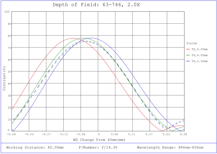
#63-746, 2X, 40mm WD CompactTL™ Telecentric Lens , Depth of Field Plot, 40mm Working Distance, f14.3
