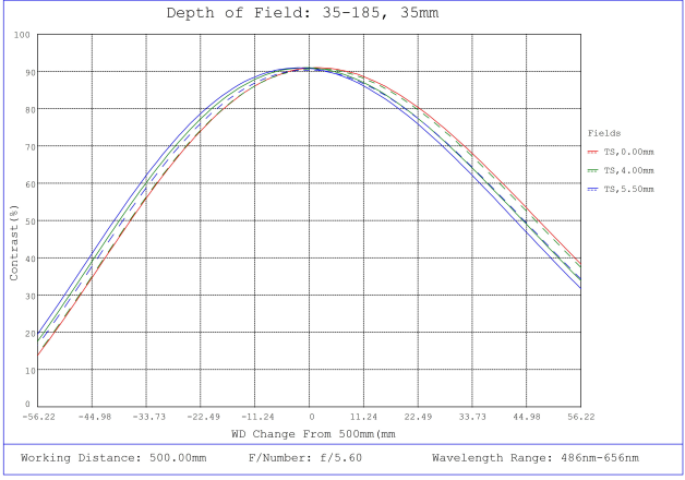
#35-185, 35mm, f/5.6 Cr Series Fixed Focal Length Lens, Depth of Field Plot, 500mm Working Distance, f5.6
