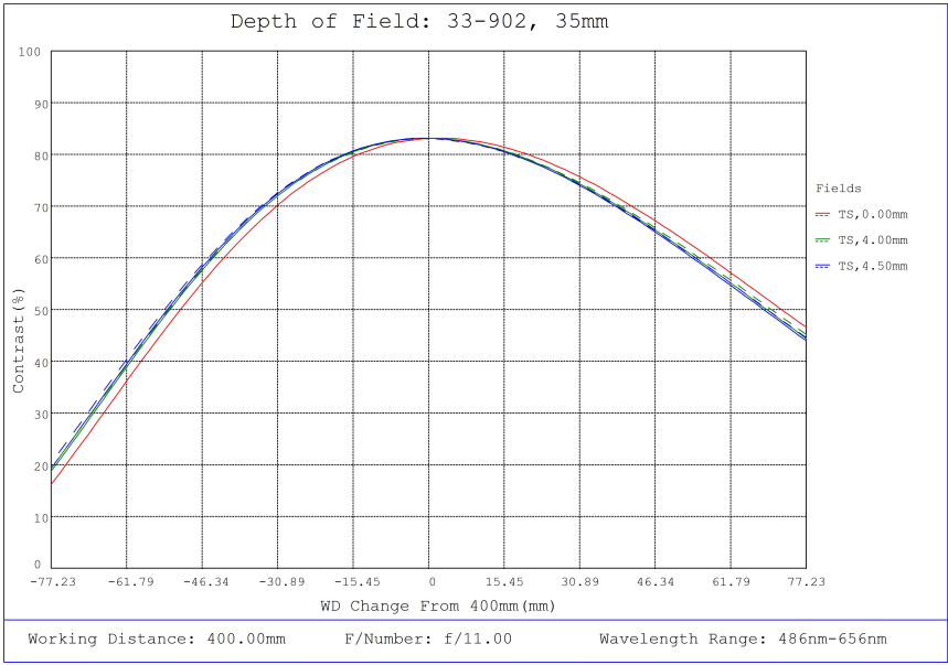
#33-902, 35mm f/11, UCi Series Fixed Focal Length Lens, Depth of Field Plot, 400mm Working Distance, f11
