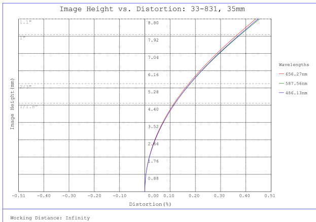
#33-831, 35mm f/4.0, HPI Series Fixed Focal Length Lens, Distortion Plot
