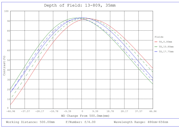
#13-809, 35mm TFL-II Mount LH Series Fixed Focal Length Lens, Depth of Field Plot, 500mm Working Distance, f4
