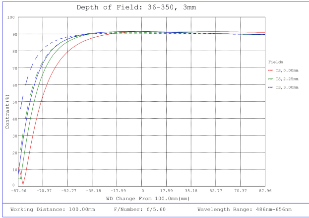
#36-350, 3mm FL f/5.6, Rugged Blue Series M12 Lens, Depth of Field Plot, 100mm Working Distance, f5.6
