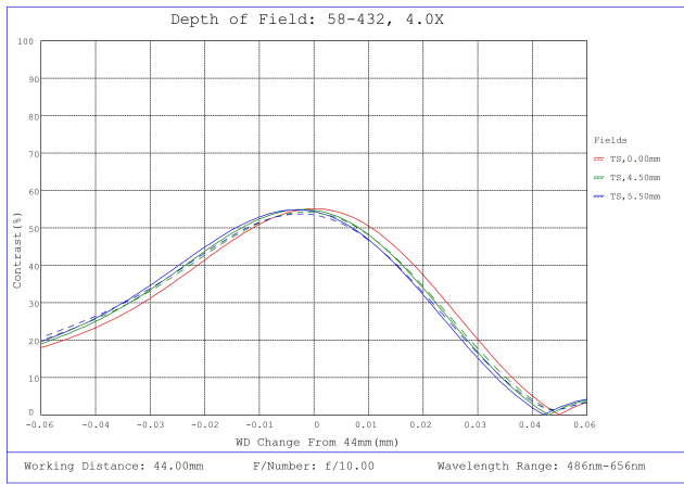
#58-432, 4.0X SilverTL™ Telecentric Lens, Depth of Field Plot, 44mm Working Distance, f10
