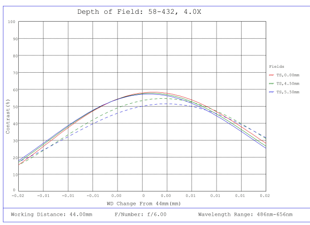
#58-432, 4.0X SilverTL™ Telecentric Lens, Depth of Field Plot, 44mm Working Distance, f6
