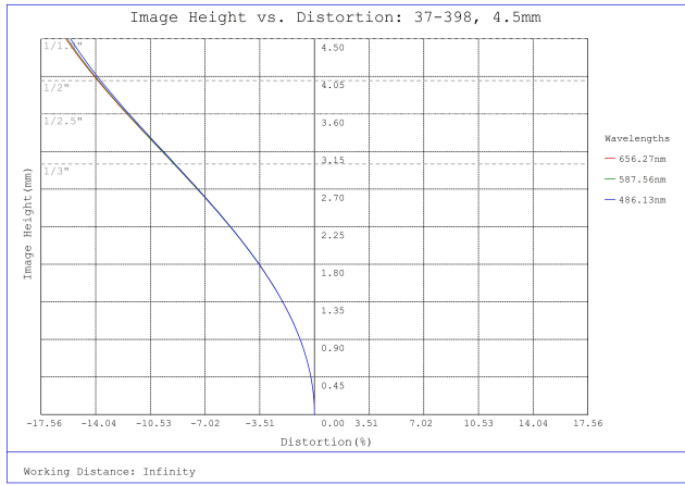
#37-398, 4.5mm, f/2 Cr Series Fixed Focal Length Lens, Distortion Plot
