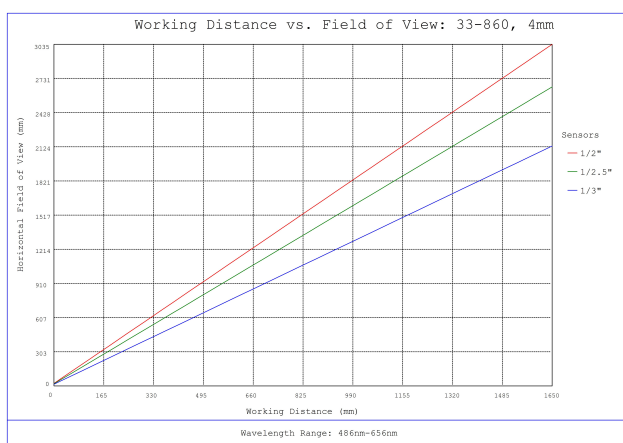
#33-860, 4mm, f/11 UCi Series Fixed Focal Length Lens, Working Distance versus Field of View Plot
