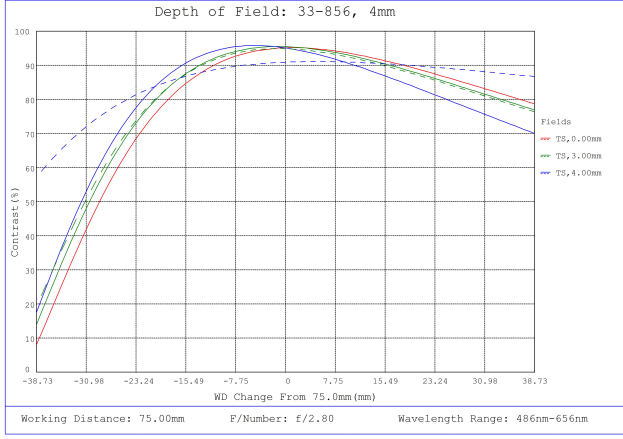
#33-856, 4mm, f/2.8 UCi Series Fixed Focal Length Lens, Depth of Field Plot, 75mm Working Distance, f2.8
