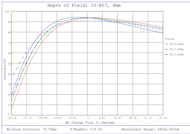
#33-857, 4mm f/4, UCi Series Fixed Focal Length Lens, Depth of Field Plot, 75mm Working Distance, f4
