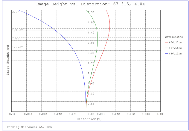
#67-315, 4X, 65mm WD, In-Line CompactTL™ Telecentric Lens, Distortion Plot
