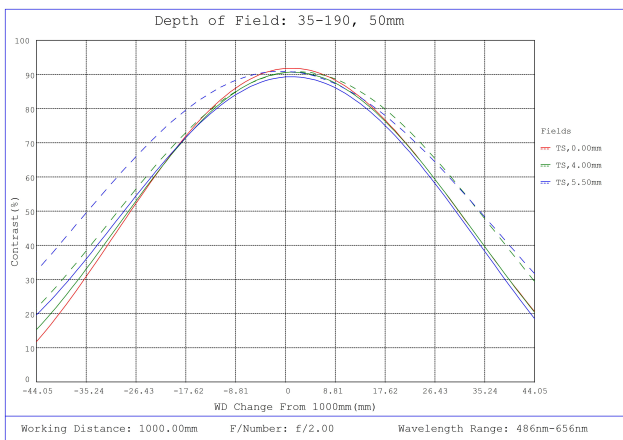
#35-190, 50mm, f/2.0 Cr Series Fixed Focal Length Lens, Depth of Field Plot, 1000mm Working Distance, f2
