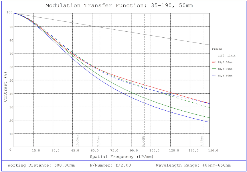
#35-190, 50mm, f/2.0 Cr Series Fixed Focal Length Lens, Modulated Transfer Function (MTF) Plot, 500mm Working Distance, f2
