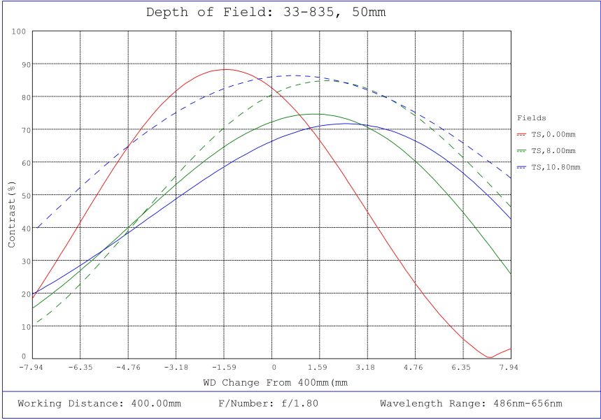
#33-835, 50mm f/1.8, HPi Series Fixed Focal Length Lens, Depth of Field Plot, 400mm Working Distance, f1.8
