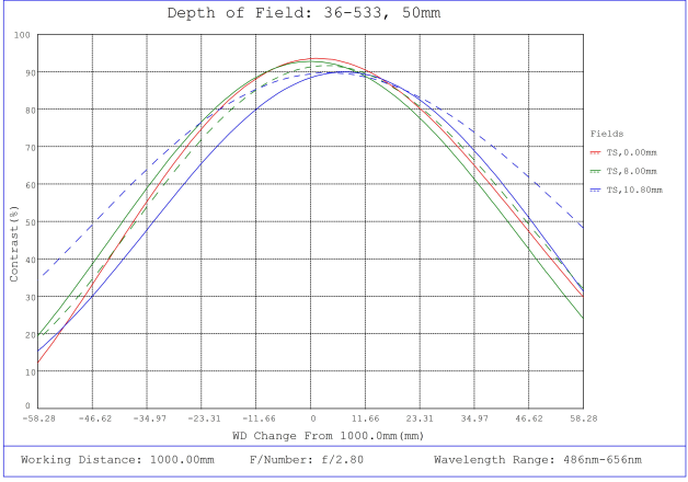
#36-533, 50mm f/2.8, HPr Series Fixed Focal Length Lens, Depth of Field Plot, 1000mm Working Distance, f2.8
