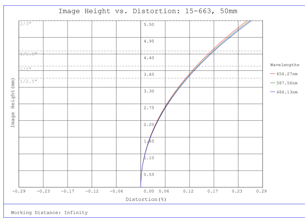
#15-663, 50mm, f/2.8 Sealed Cw Series Fixed Focal Length Lens, Distortion Plot
