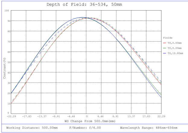
#36-534, 50mm f/4.0, HPr Series Fixed Focal Length Lens, Depth of Field Plot, 500mm Working Distance, f4
