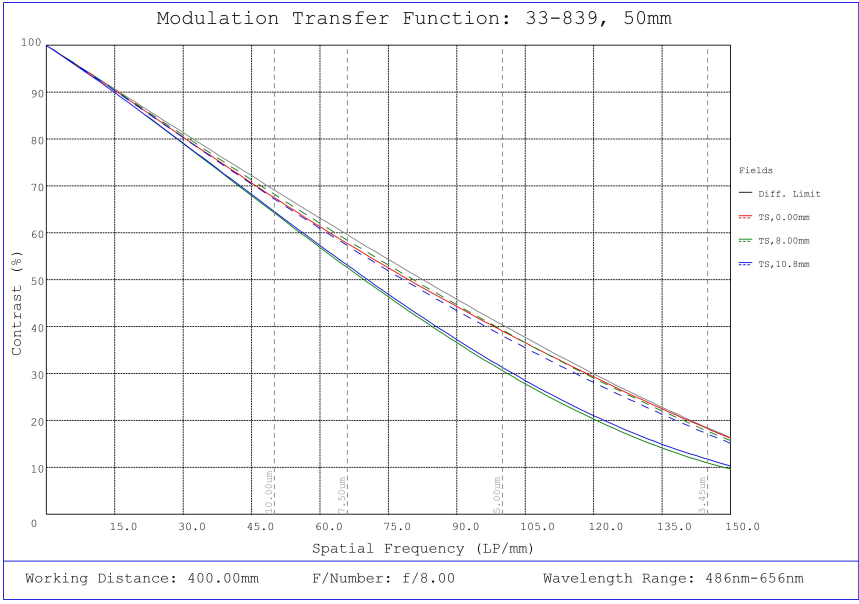
#33-839, 50mm f/8.0, HPI Series Fixed Focal Length Lens, Modulated Transfer Function (MTF) Plot, 400mm Working Distance, f8
