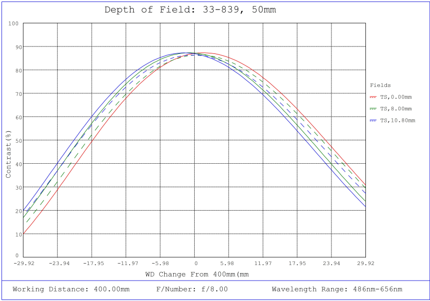
#33-839, 50mm f/8.0, HPI Series Fixed Focal Length Lens, Depth of Field Plot, 400mm Working Distance, f8
