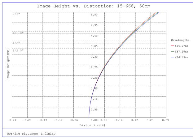
#15-666, 50mm, f/8.0 Sealed Cw Series Fixed Focal Length Lens, Distortion Plot
