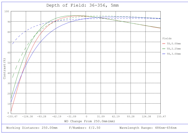
#36-356, 5mm FL f/2.5, Rugged Blue Series M12 Lens, Depth of Field Plot, 250mm Working Distance, f2.5
