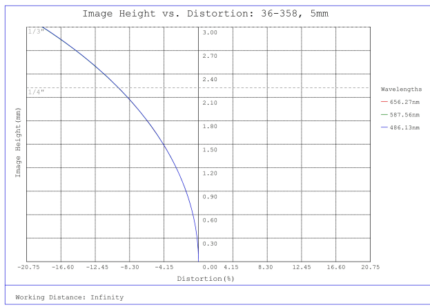
#36-358, 5mm FL f/5.6 , Rugged Blue Series M12 Lens, Distortion Plot
