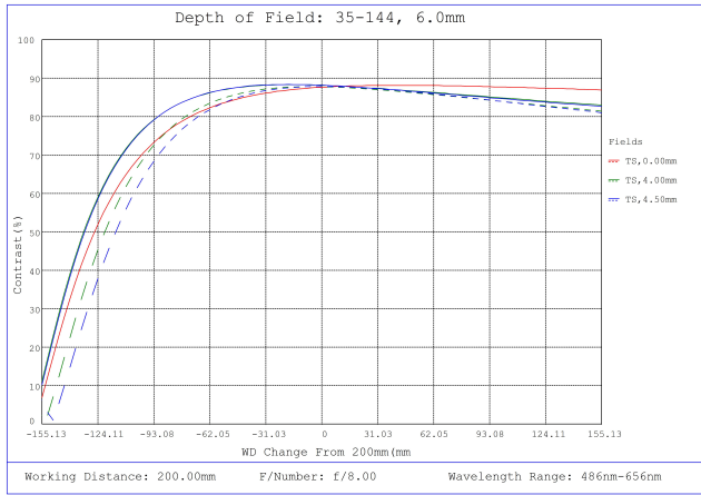
#35-144, 6mm, f/8 Cr Series Fixed Focal Length Lens, Depth of Field Plot, 200mm Working Distance, f8
