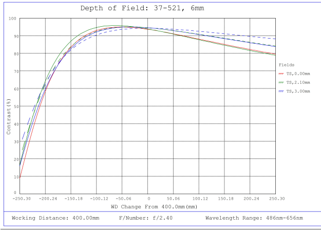
#37-521, 6mm FL, Liquid Lens M12 Lens, Depth of Field Plot, 400mm Working Distance, f2.4
