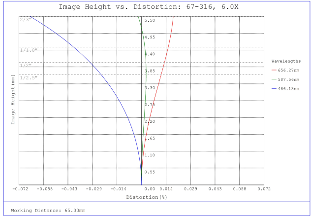
#67-316, 6X, 65mm WD, In-Line CompactTL™ Telecentric Lens, Distortion Plot
