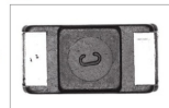
A Ring Light can illuminate the electrode part evenly and make an image.
