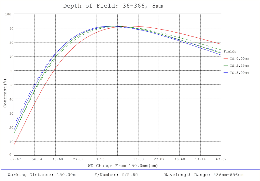
#36-366, 8.0mm FL f/5.6 Rugged Blue Series M12 Lens, Depth of Field Plot, 150mm Working Distance, f5.6
