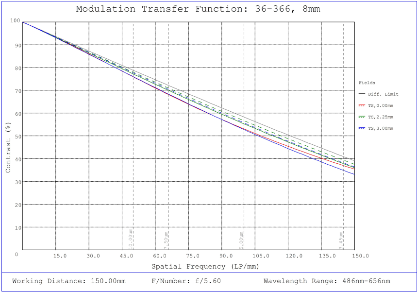
#36-366, 8.0mm FL f/5.6 Rugged Blue Series M12 Lens, Modulated Transfer Function (MTF) Plot, 150mm Working Distance, f5.6
