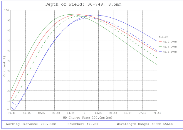
#36-749, 8.5mm f/2.8, 75mm-∞ Primary WD, HRi Series Fixed Focal Length Lens, Depth of Field Plot, 200mm Working Distance, f2.8
