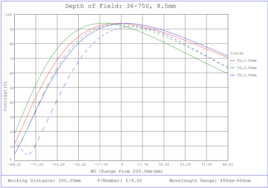
#36-750, 8.5mm f/4, 75mm-∞ Primary WD, HRi Series Fixed Focal Length Lens, Depth of Field Plot, 200mm Working Distance, f4
