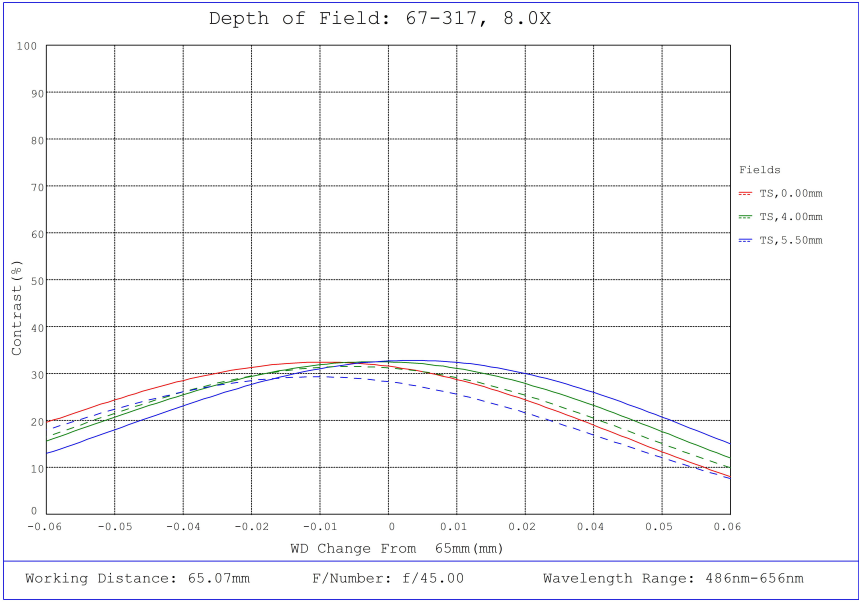
#67-317, 8X, 65mm WD, In-Line CompactTL™ Telecentric Lens, Depth of Field Plot, 65mm Working Distance, f45
