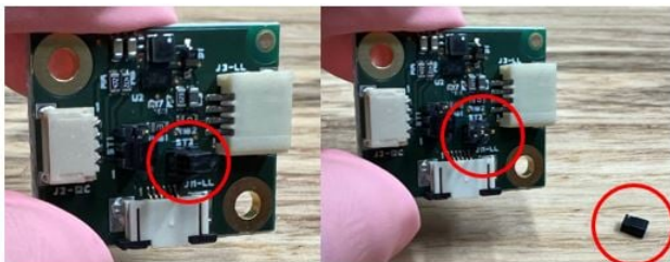
Jumper at ST2 installed
