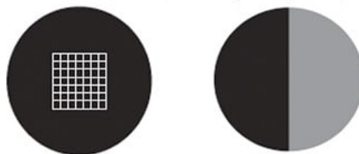
7 x 7 Grid Reticle (#88-521) Edge Reticle (#88-522)
