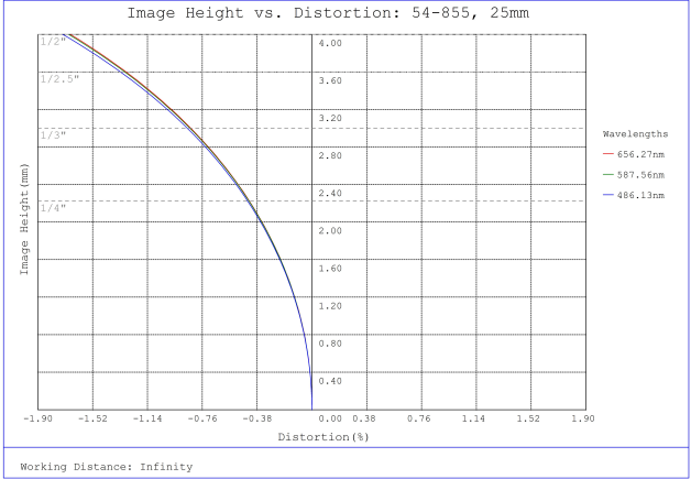
#54-855, f/2.1, 25mm Focal Length Green Series M16 Lens, Distortion Plot
