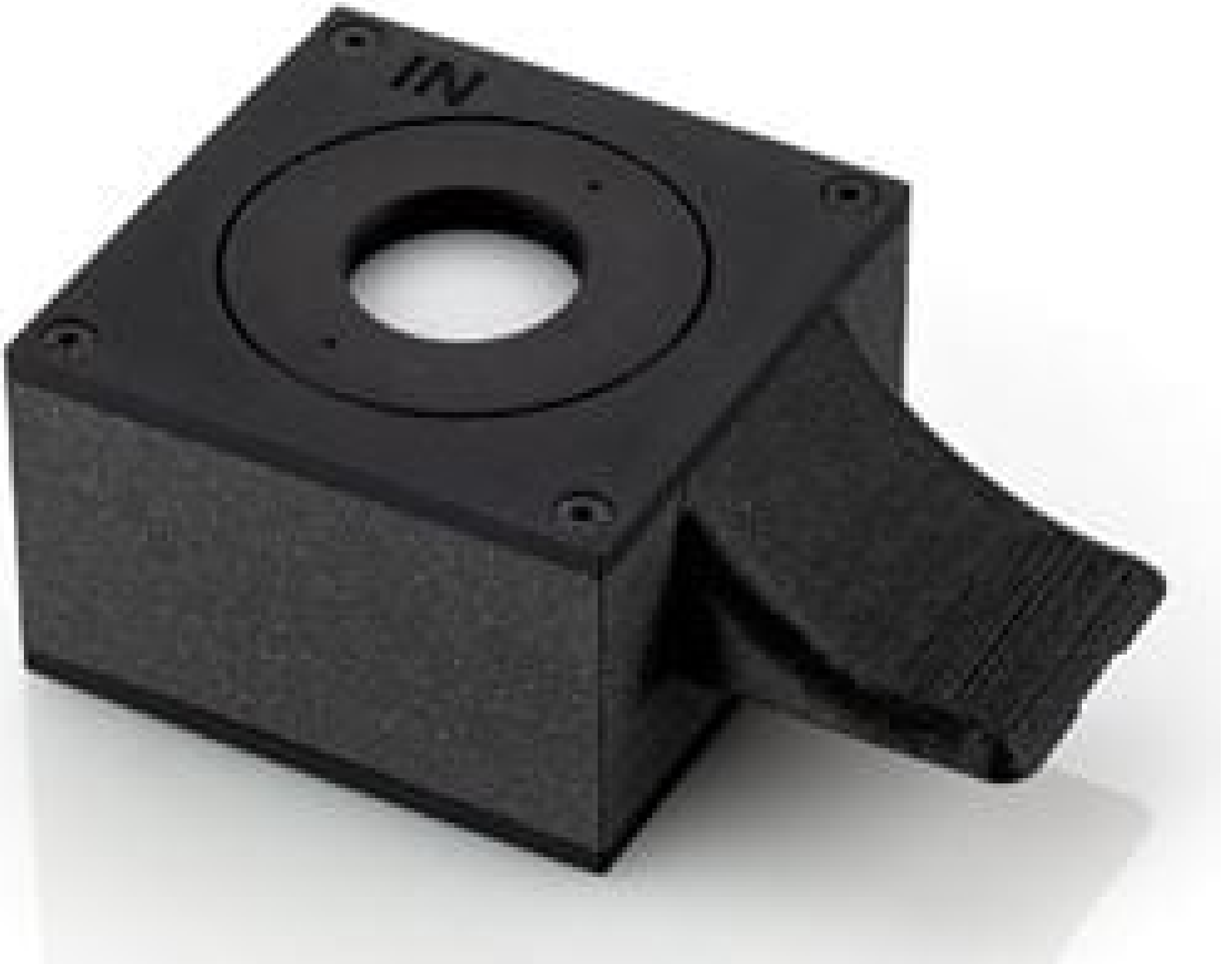
fNIRS Standard Phantom - IEC 80601-2-71
