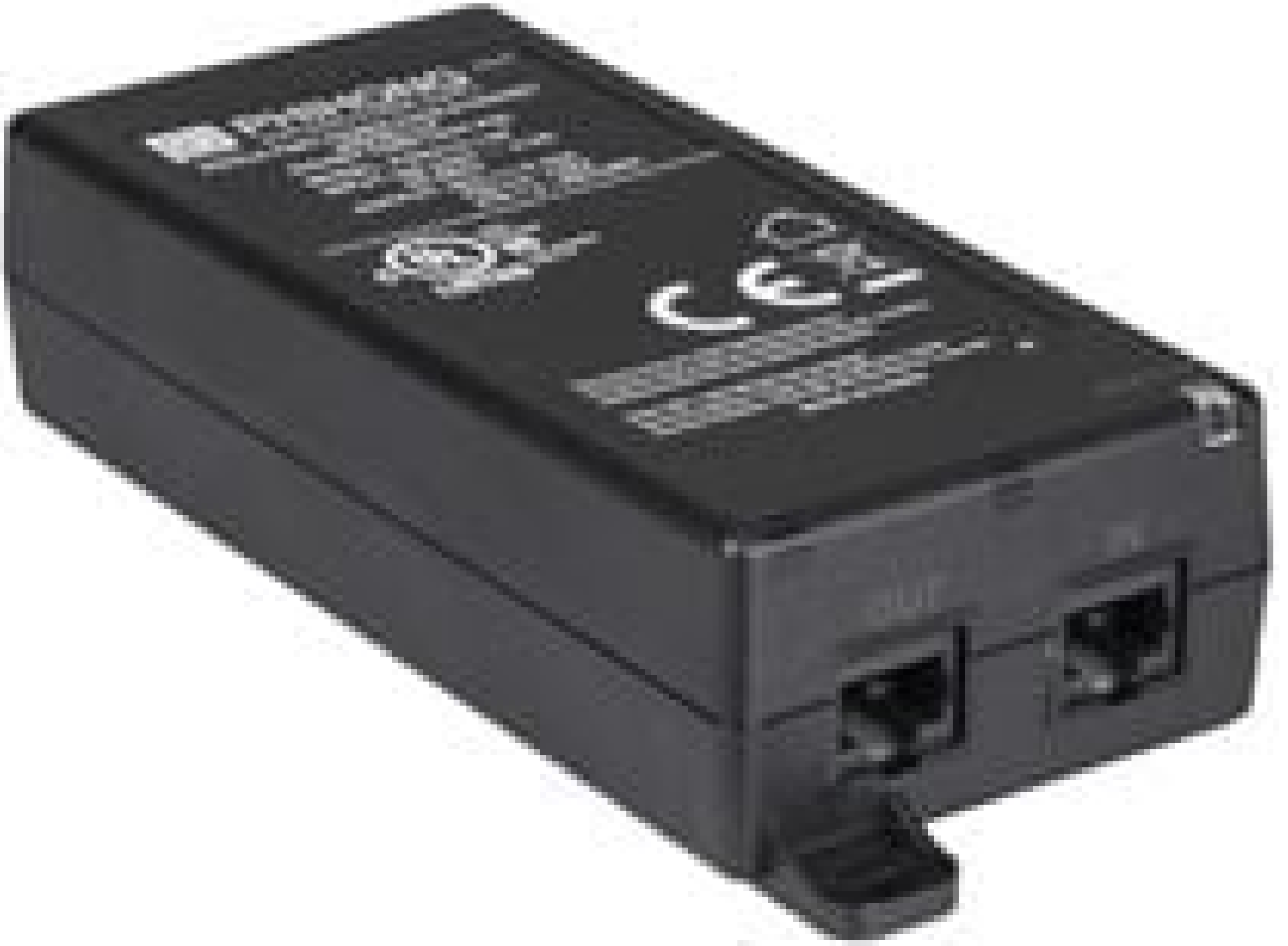
Power Over Ethernet (PoE) Single Port injector, #68-469 (pictured without required power supply)
